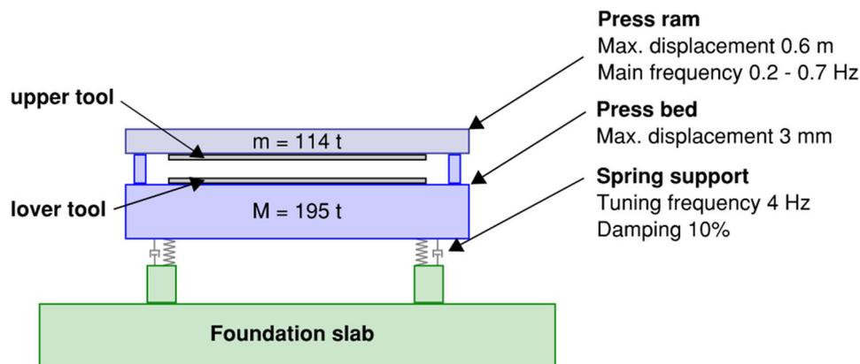
Figure 1.1 Schematic presentation of a press machine
