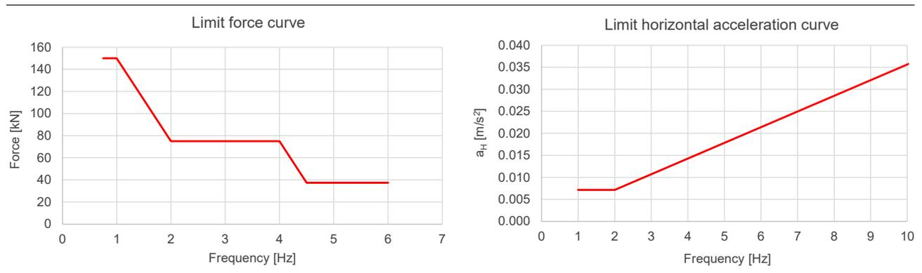
Figure 6.1 Force and acceleration limit curves in frequency domain
