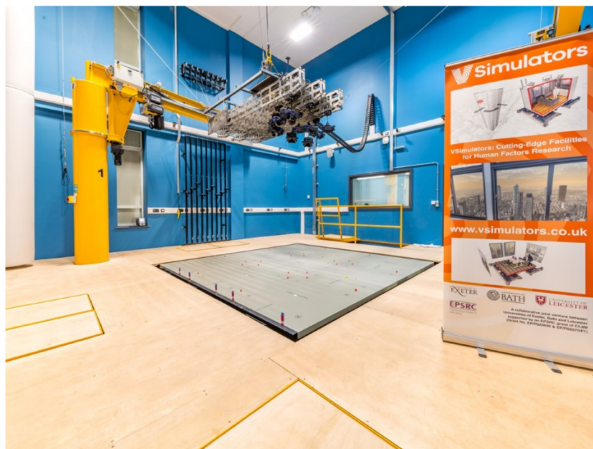
Figure 2: VSimulator rigid platform within an 8 m cube purposely built to accommodate the facility built by The University of Exeter at Exeter Science Park.
