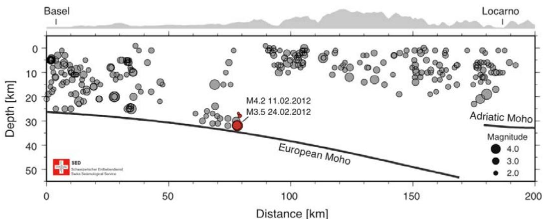
Figure 2: Depth cross-section from Basel to Locarno showing seismicity from 1985-2012 (grey circles) as recorded by the SED. The M4.2 mainshock of February 11, 2012, and its three aftershocks are marked by red circles. Only earthquakes within a swath of  $\pm 50$  km of the profile and with well constrained focal depths are shown.
