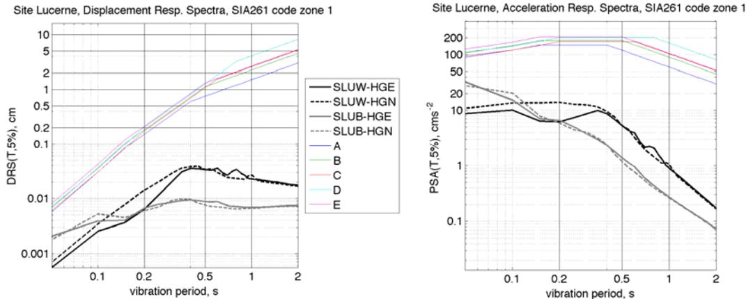
Figure 8: Response spectra (left: acceleration; right: displacement) in Lucerne compared to SIA261 (zone 1) design code for the A, B, C, D and E subsoil classes.
