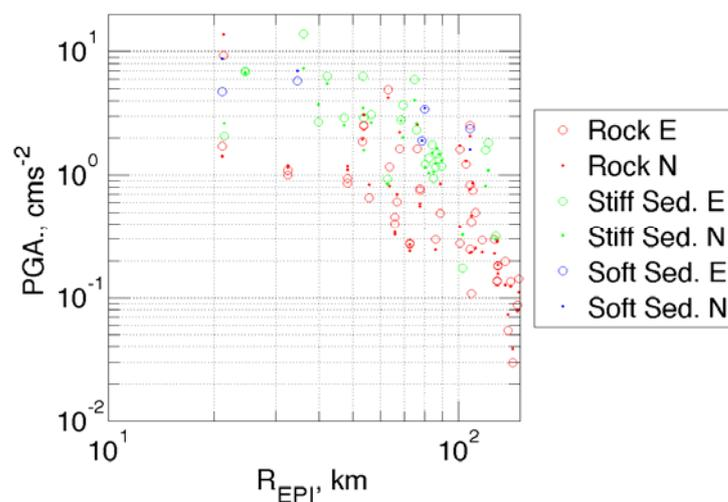
Figure 4: Attenuation of horizontal PGA values as a function of epicentral distance (East and North components).
