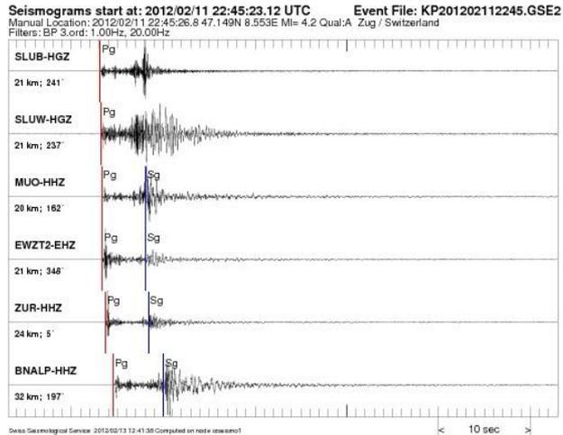
Figure 1: Some recordings used to locate the earthquake hypocenter. The red mark depicts the onset of the P-waves, the blue mark depicts the onset of the S-waves.
